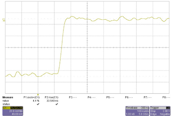
Fig. 3. Rise time of the charge preamplifier corresponding to an output signal produced by pulsing the first ring of the SDD. The measured rise time, of about 30 ns, is therefore limited by the preamplifier itself and not by the drift/collection properties of the charge inside the SDD.
