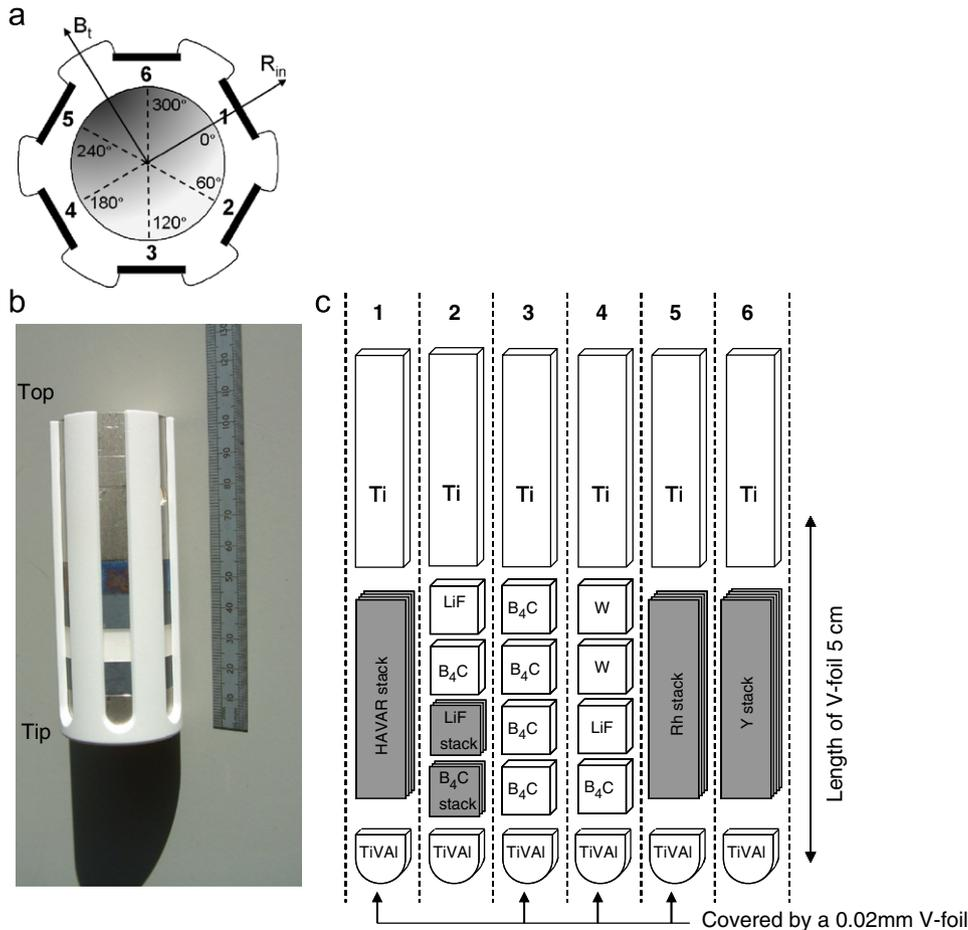
**Fig. 1.** (a) Cross-section of the probe and its orientation with respect to the toroidal magnetic field ( $B_t$ ) and the major radius of the Tokamak ( $R_{in}$ ), (b) picture of the BN activation probe and (c) schematic diagram of the sample layout. The numbers in (a) and (c) indicate the six slots where the samples were placed.
