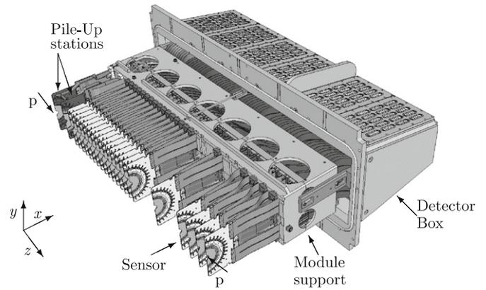
**Fig. 2.** Overview of the VELO left half. The sensors, module supports and detector box are indicated.
