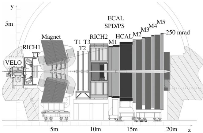
**Fig. 1.** The LHCb detector setup with the different sub-detectors in the longitudinal plane. The Vertex Locator is shown on the left-hand side of the diagram and the other sub-detectors of the spectrometer are indicated.
