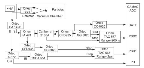
Fig. 1. The experimental setup. CFD (Constant Fraction Discriminator); TSCA (Timing Single-Channel Analyzer); TAC (Time-to-Amplitude Converter); ADC (Analog-to-Digital Converter).
