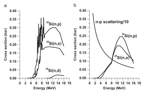
Fig. 2. The corresponding cross-sectional data from ENDF/B-VII.0 [10]. (a) Neutron induced reactions on <sup>28</sup>Si; (b) neutron induced reactions on <sup>29</sup>Si and n-p scattering (divided by a factor of 10).
