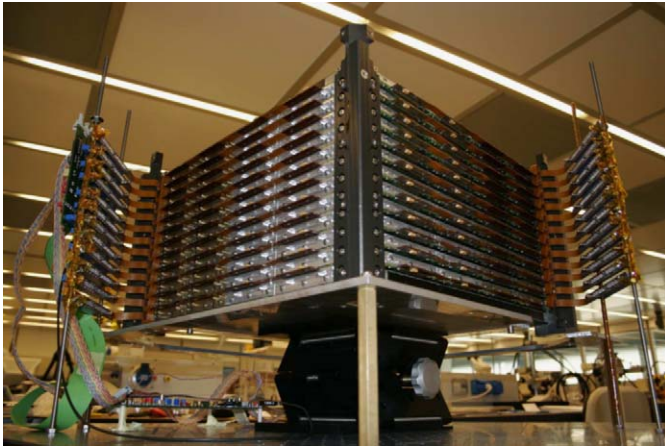
Fig. 1. Photo of the tracker before the assembly of the 2 front-end boards (June 2005).
