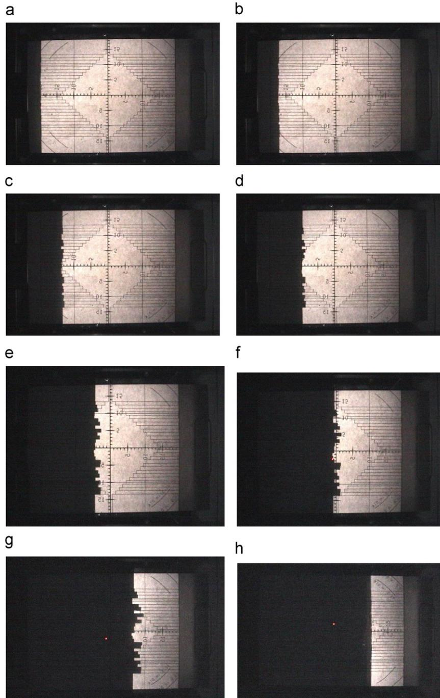
**Fig. 1.** Images (a)–(h) show the sequence of Siemens Primus Linac X1 MLC leaves bank motion images at collimator and gantry angle of  $90^\circ$  with the MLC check tray overlaid onto the leaves shadow.
