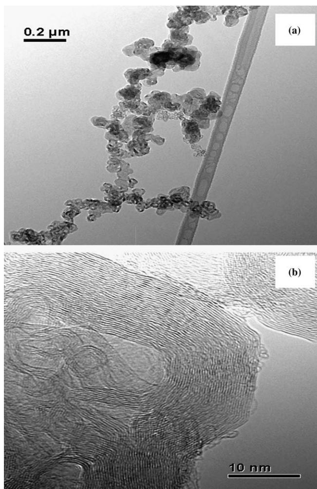
Fig. 1. Transmission electron micrographs of PUREBLACK<sup>®</sup> Carbon: (a) low magnification showing the chain structure and (b) high magnification showing well defined graphene layers of its graphitic structure (courtesy: Superior Graphite/Columbian Chemicals Co.).
