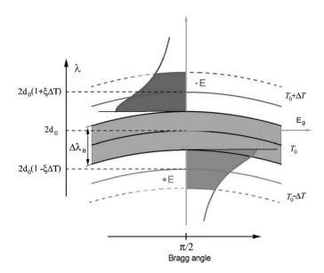
Fig. 1. Electric field for neutrons close to the Bragg condition (Bragg angle  $\pi/2$  and  $\lambda=2d_0$ ) in a non-centrosymmetric crystal: the electric field has a pole for neutrons exactly fulfilling the Bragg condition. By choosing the deviation from the Bragg condition, value and sign of the electric field can be selected. We use Bragg reflection in a second crystal with a different temperature  $T_0\pm\Delta T$  to select neutrons with a certain deviation.
