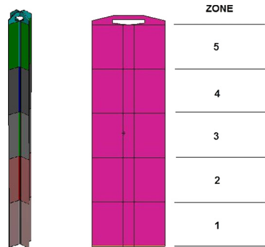
Fig. 2. Axial division cells of the model.
