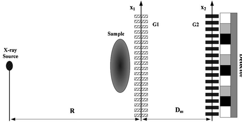
**Fig. 1.** Schematic representation of grating-based phase-contrast imaging setup. G1 is a phase grating or an amplitude grating while G2 must be an absorption grating. Both gratings have a duty cycle of 0.5.
