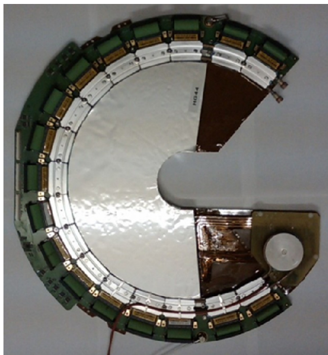
Fig. 2. GEM chamber assembled with its horseshoe shaped readout card.
