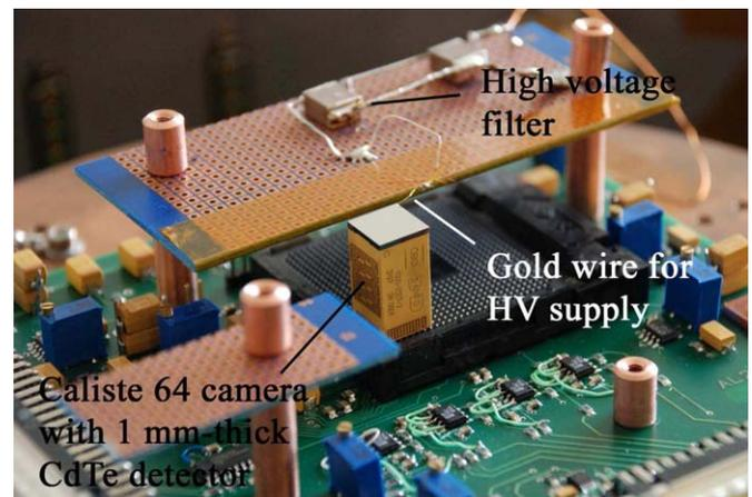
**Fig. 2.** Caliste 64 camera in the thermal enclosure of the test bench. High voltage is supplied by a  $100 \mu\text{m}$  gold wire glued on the planar cathode of the 1-mm-thick detector. A (non-visible) plate with an aperture is placed above the camera to receive the Am source.
