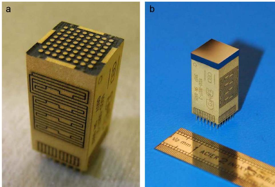
**Fig. 1.** (a)  $10 \times 10 \times 18 \text{ mm}^3$  electrical body of Caliste 64, featuring four ASIC IDeF-X V1.1 responsible for reading out two rows of 8 pixels each. (b) Caliste 64 camera with a 2-mm-thick Schottky CdTe detector of 64 pixels.
