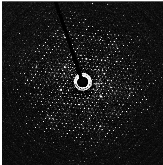
Fig. 2. Electron diffraction pattern from two-dimensional crystals of bacteriorhodopsin recorded on a CCD camera [3] at 120 keV.
