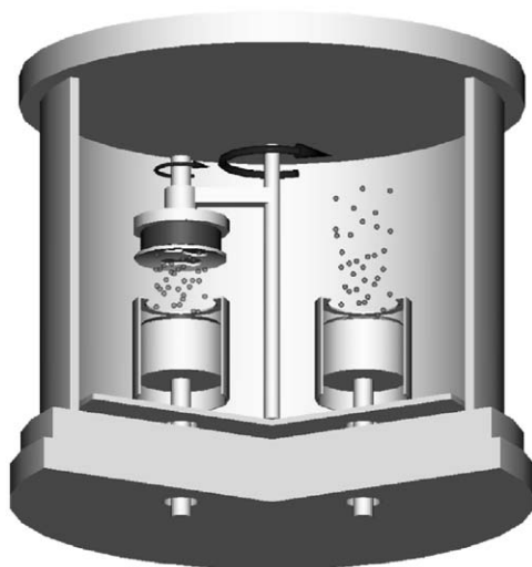
Fig. 1. Scheme of the correction procedure by the vacuum deposition thin films through a mask.
