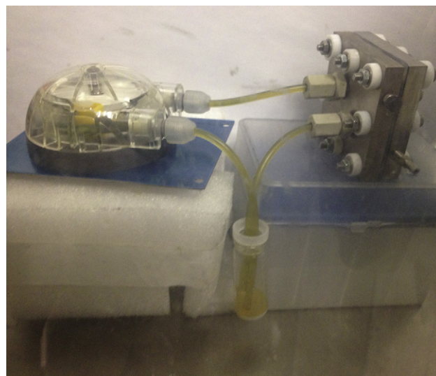
Fig. 2. Experimental setup of the half-cell RFLB system.
