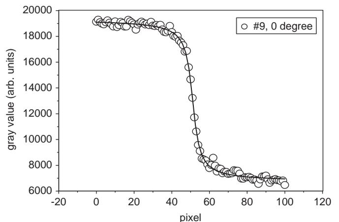
**Fig. 1.** Sample to explain the mathematics process with edge-spread function, converter #9, angle of the turntable = 0°.
