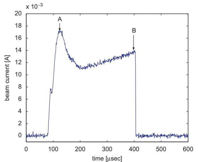
Fig. 2. Plot of the beam current vs. time of a  $330\mu s$  long unchopped beam pulse. The points A and B indicate where the phase scan data are taken, which is displayed in Fig. 3. The point A (B) is 50 ( $330\mu s$ ) from the beginning of the beam pulse. This beam current was provided by ion source used then. Lately the SNS linac has routinely delivered beam with peak current of about 38 mA.
