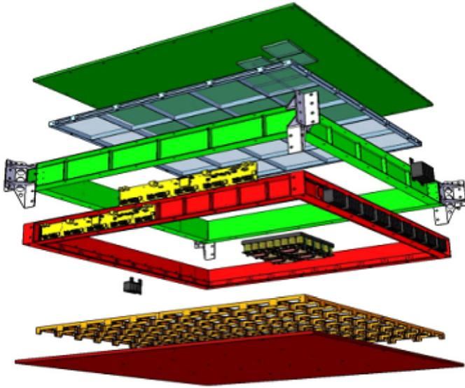
Fig. 1. Exploded CAD view of the CHERCAM mechanical structure.
