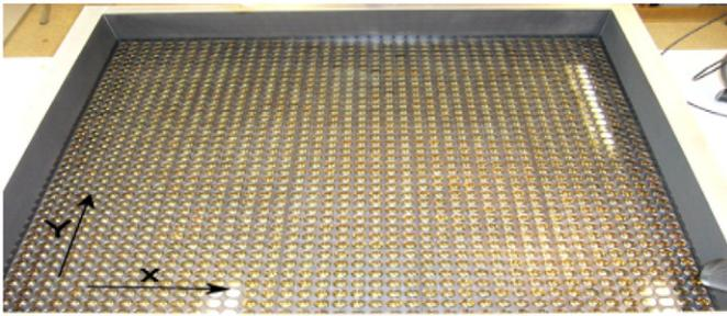
Fig. 2. Aerogel radiator plane of the CHERCAM detector: 40 × 40 PMTs in a 1.1 m × 1.1 m plane.
