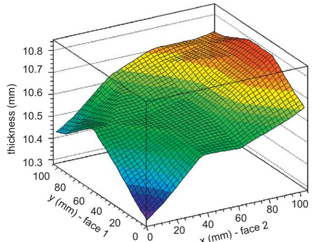
Fig. 3. Thickness variation in SP50 aerogel tiles.
