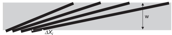
Fig. 5. Compact arrangement of the monochromator mirrors taking into account the finite thickness of the silicon substrates.
