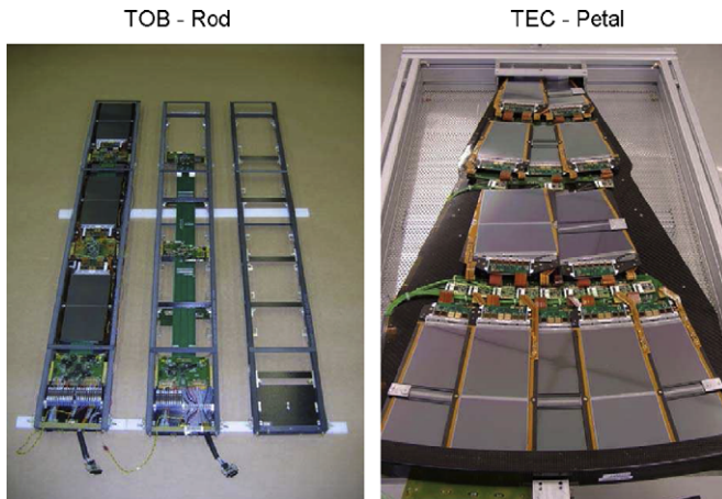
Fig. 3. Carbon fiber support structures for TOB and TEC: (left) a rod in three different phases of construction; (right) a fully assembled petal.
