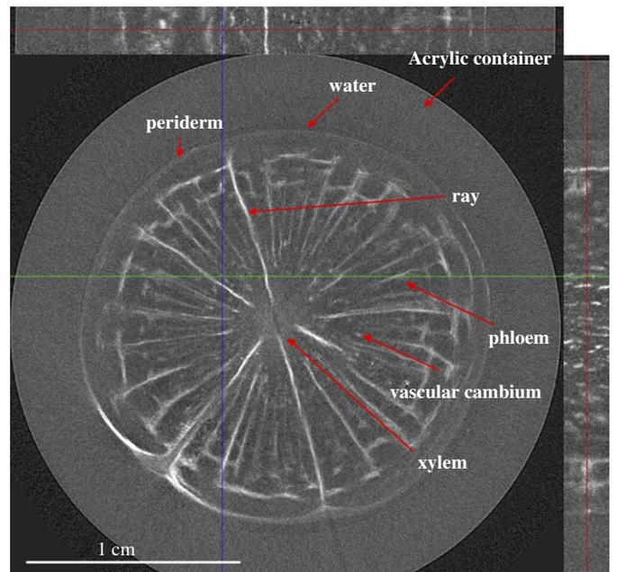
Fig. 2. DEI-CT of a carrot. The top and right images show tangential cross-sections. The center image shows the axial view. Brighter color corresponds to larger apparent absorption.
