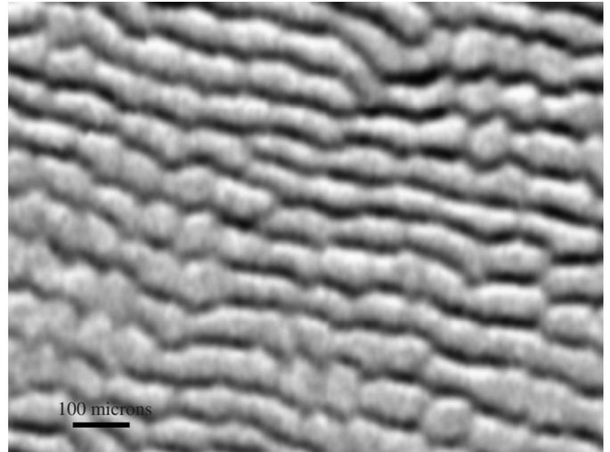
Fig. 1. DEI planar radiograph at 20 keV, 333 analyzer. Darker grayscale corresponds to less X-ray intensity, or more apparent absorption.
