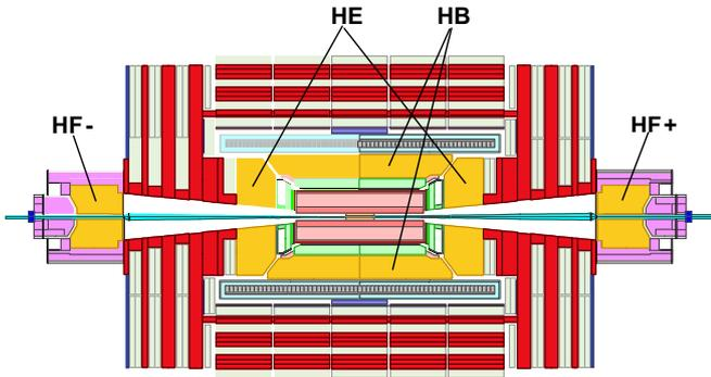
Fig. 1. Three subdetectors make up the hadronic calorimeter system in CMS—Hadronic Barrel (HB), Hadronic Endcap (HE) and Hadronic Forward (HF).
