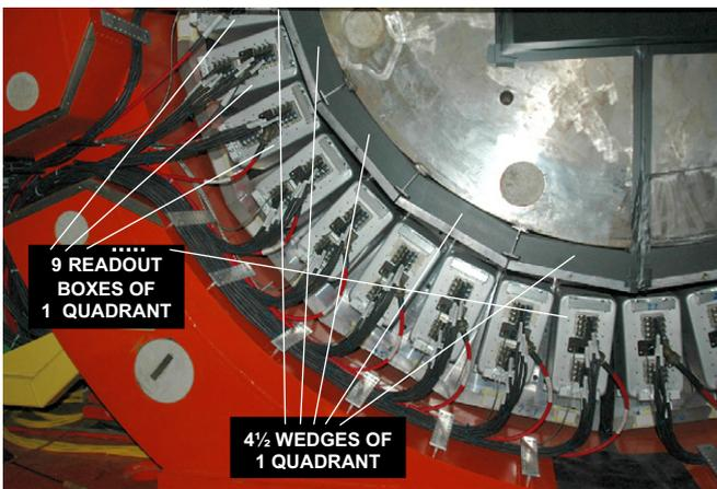
Fig. 2. Back view of one quadrant (a 90° section) of the calorimeter with its 4½ wedges and nine readout boxes.
