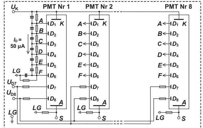
Fig. 3. Electrical diagram of the PMT parallel voltage distribution showing that there are three voltages provided to PMTs in a group of eight—the photocathode is set at  $U_K$  and the last two dynodes are set at  $U_{D7}$  and  $U_{D8}$ , respectively.
