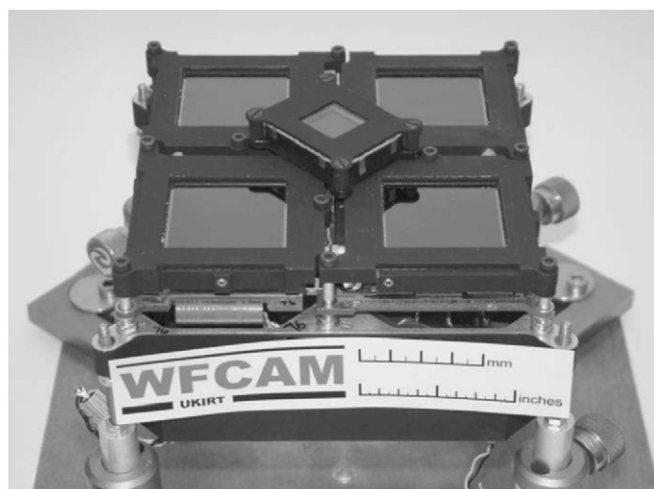
Fig. 3. WFCAM focal plane mosaic.
