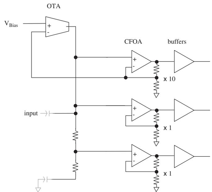
Fig. 2. Circuit principle. The external components (capacitors) are represented in gray.
