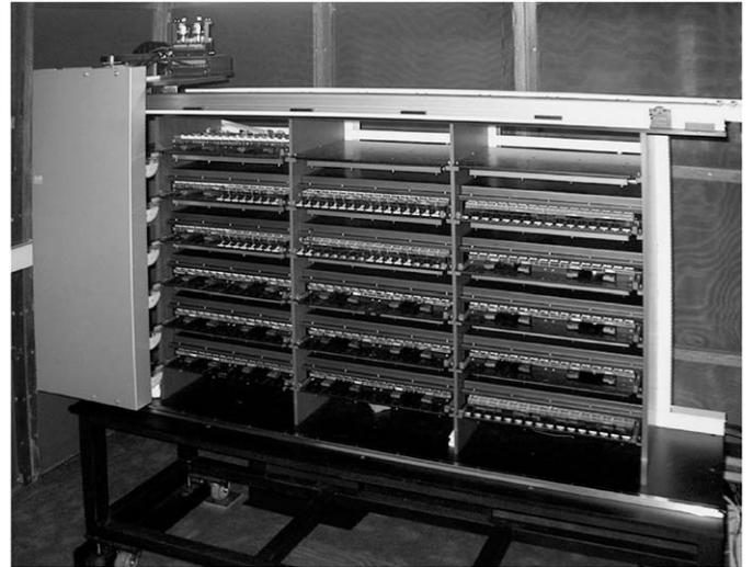
Fig. 3. The CMS ECAL photodetection capsule test bench.
