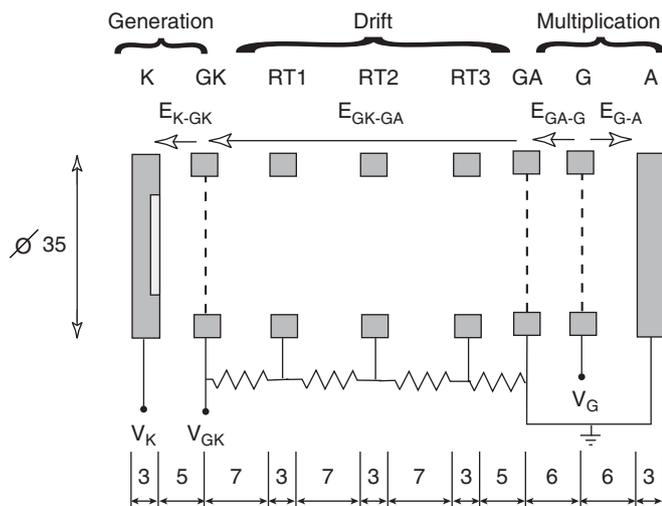
Fig. 1. Schematic view of the detector. Numbers represent the dimensions in mm. Electrical scheme of the connections and electric field directions are also shown.
