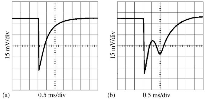
Fig. 2. (a) Photocathode signal waveform when the device operates as an ionization chamber ( $p_{\text{Ar}} = 10 \text{ mbar}$ ;  $T \sim 300 \text{ K}$ ). (b) Photocathode signal waveform at the same pressure and temperature conditions, when the device operates as a proportional chamber.
