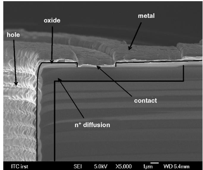
Fig. 1. SEM micrograph showing a detail of a 3D-stc device.
