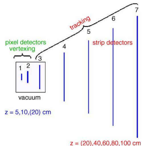
Fig. 2. Configuration of the Silicon Tracking System for a conceptual design study. Two detector regions focussing on tracking and vertexing are indicated.
