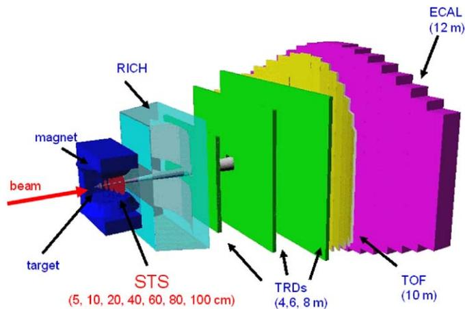
Fig. 1. The concept of the CBM experiment: charged particle tracking exclusively in a Silicon Tracking System (STS), in a compact magnetic field directly behind the target. Particle identification downstream of the magnet in ring imaging Cherenkov counters (RICH) and transition radiation detectors (TRDs), together with a time-of-flight (TOF) measurement, and electromagnetic calorimetry (ECAL). A dedicated muon identification system is under study.
