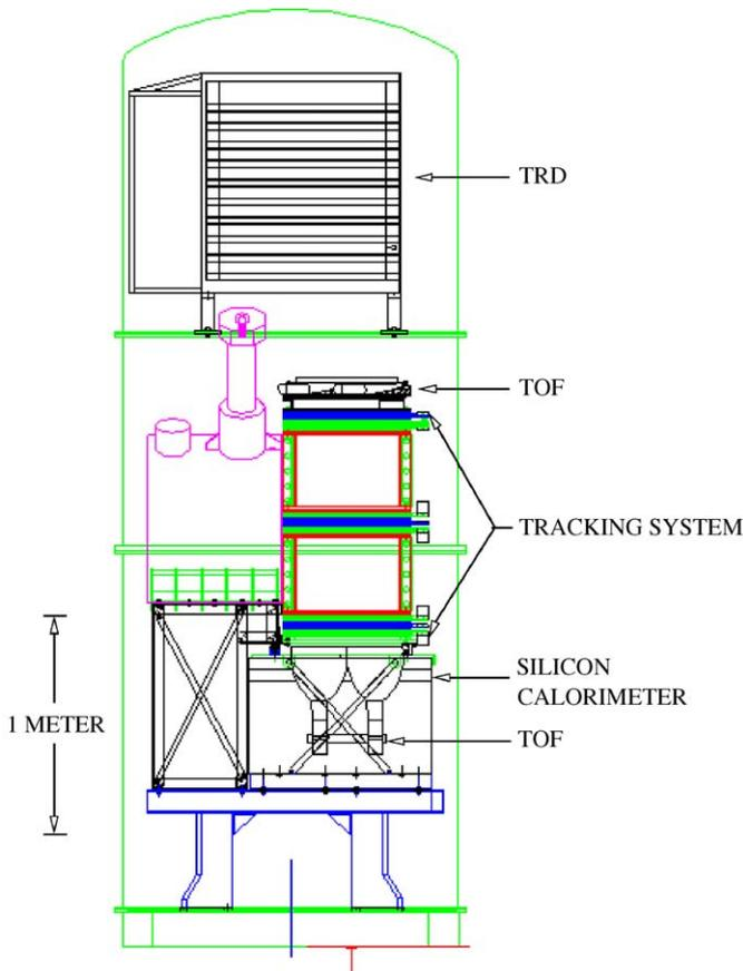
Fig. 1. Schematic diagram of TS93-experiment [8].
