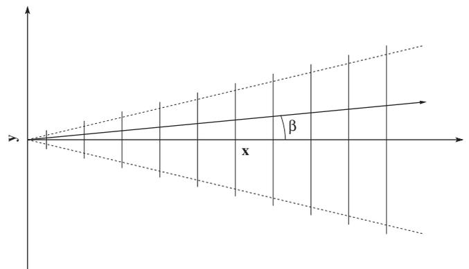
Fig. 2. A detector geometry consisting of 10 parallel detector planes.
