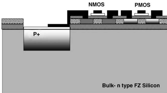
Fig. 1. The idea of the fully depleted active pixel sensor manufactured in SOI technology.
