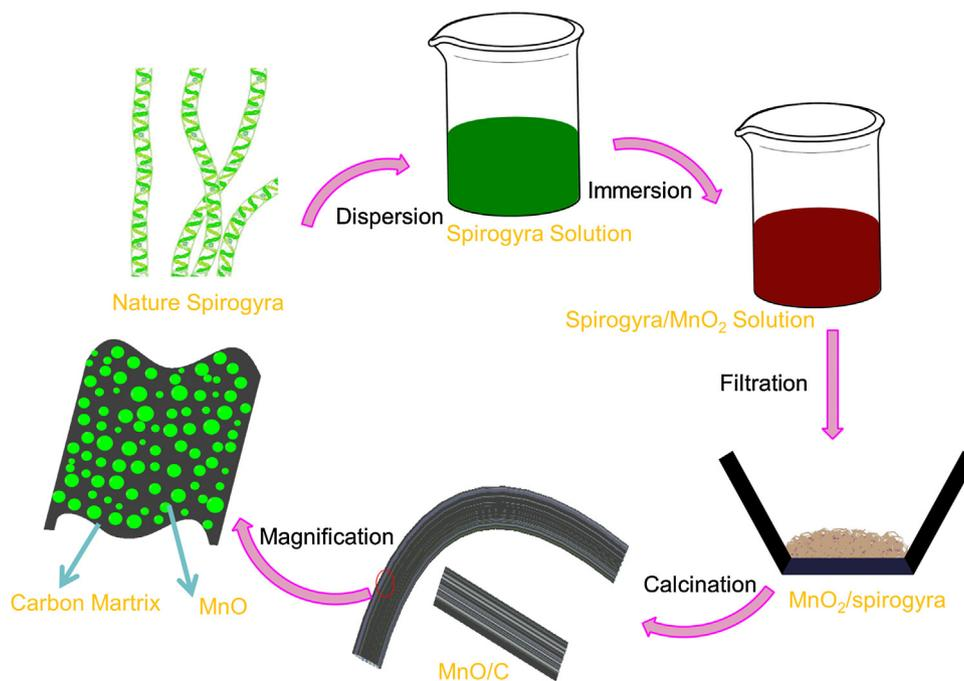
Fig. 1. Schematic illustration of the fabrication process of spirogyra-templated MnO/C microtubes.
