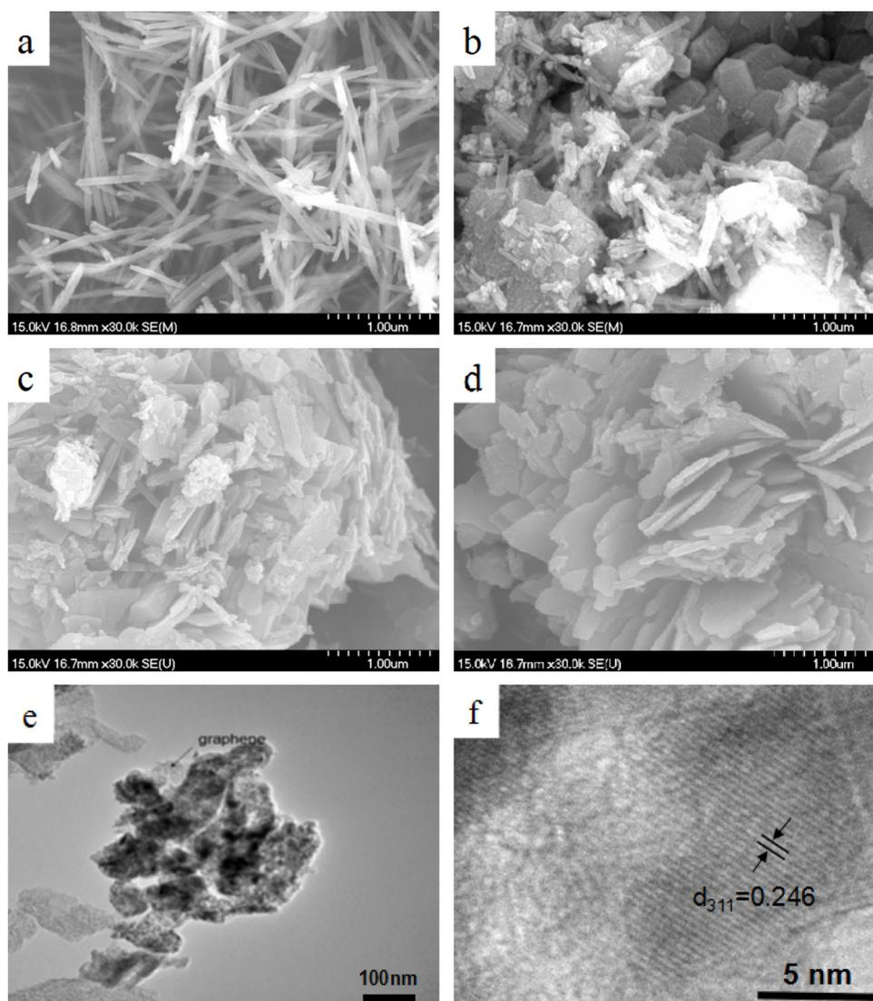
**Fig. 1.** The SEM images of metal oxide/rGO composites after 300 °C calcination CMOG1, b) CMOG2, c) CMOG3, d) CMOG5 (e) TEM, (f) HRTEM images of the CMOG5 composite.
