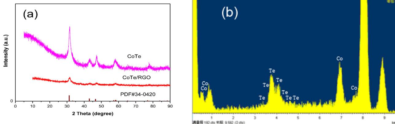
Fig. 1. (a) XRD and (b) EDS patterns of cobalt telluride.
