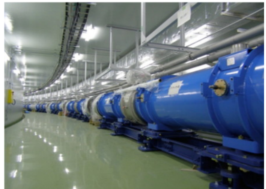
Figure 3: The neutrino beam line. Blue tanks have superconducting magnets.
