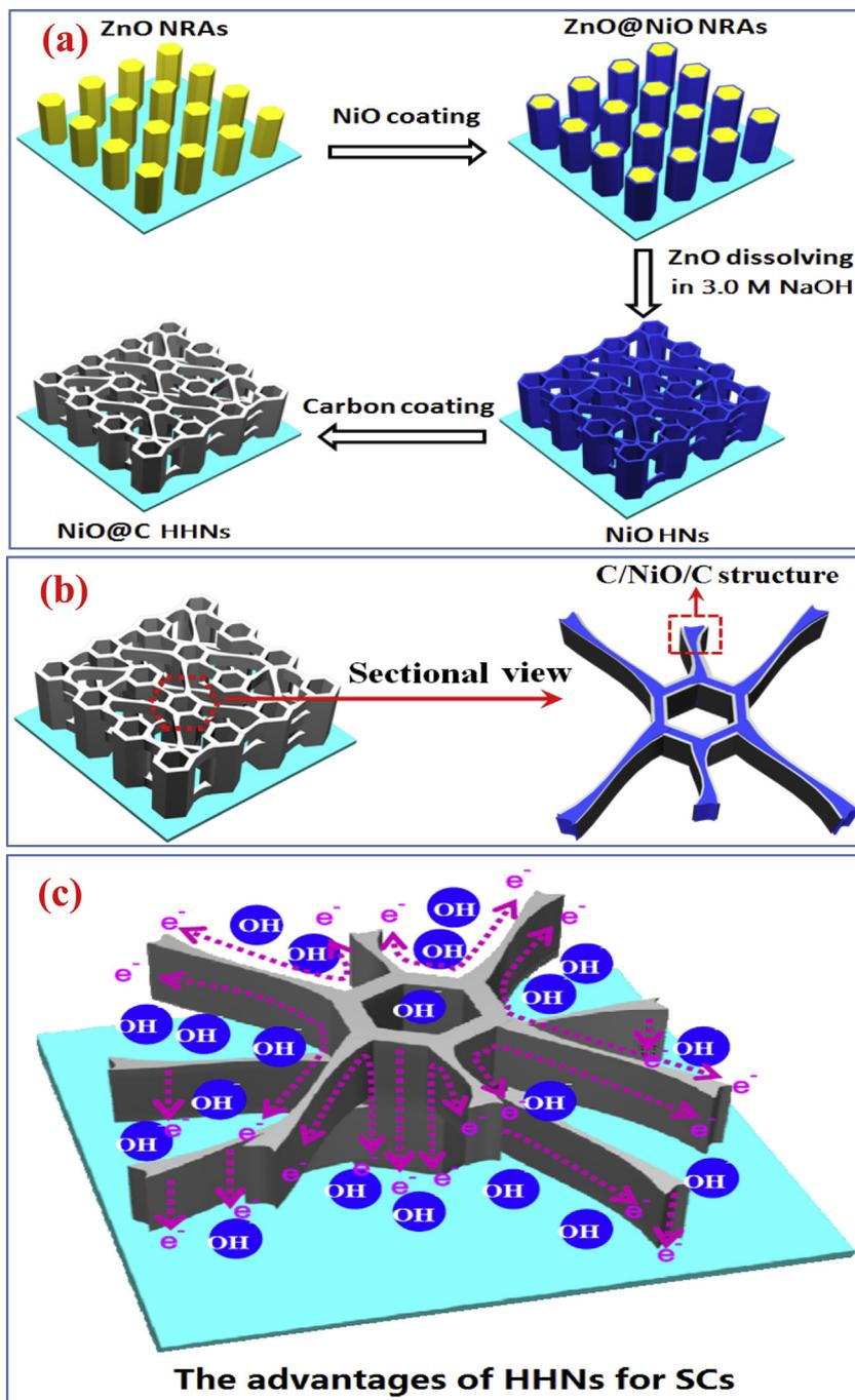
**Scheme 1.** (a) Schematic illustration of the fabrication process of NiO@C HHNs; (b) Sectional view of NiO@C HHNs; (c) The advantages of NiO@C HHNs for SCs: large surface area and fast transports of ions and electrons.
