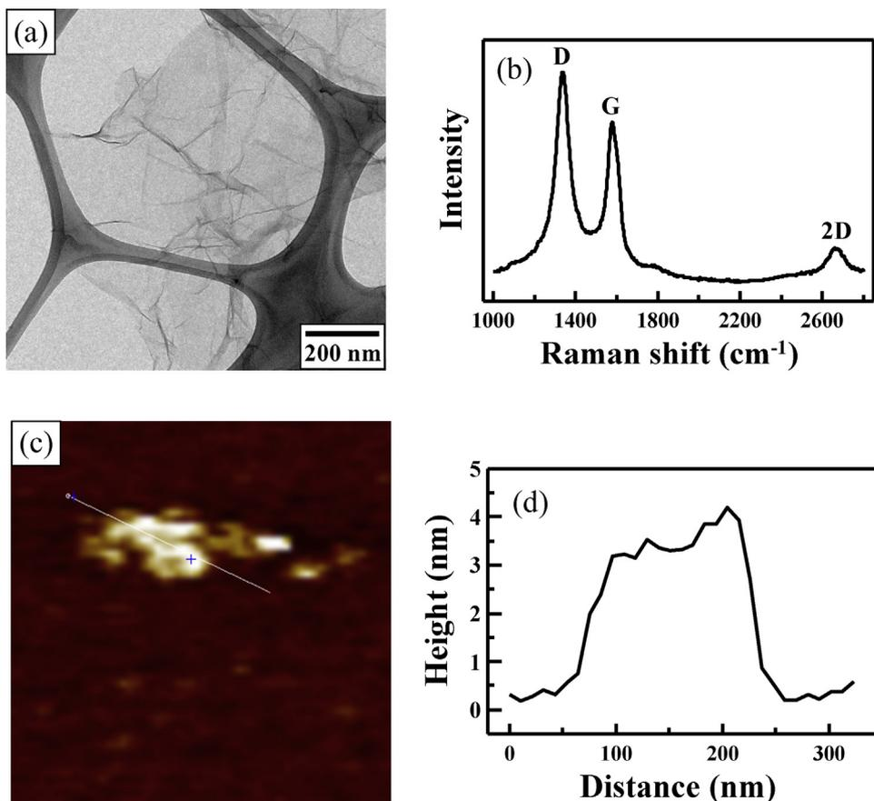
**Fig. 1.** (a) TEM image, (b) Raman spectrum, (c) AFM image, and (d) height profile across the marked line in (c) of synthesized GNSs.
