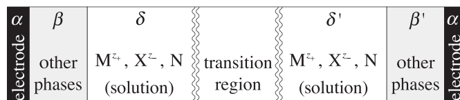
Fig. 1. Schematic drawing of a general electrolytic cell containing a binary electrolytic solution.
