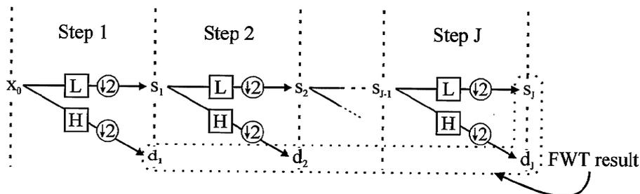
Fig. 1. General scheme of the FWT algorithm [8].
