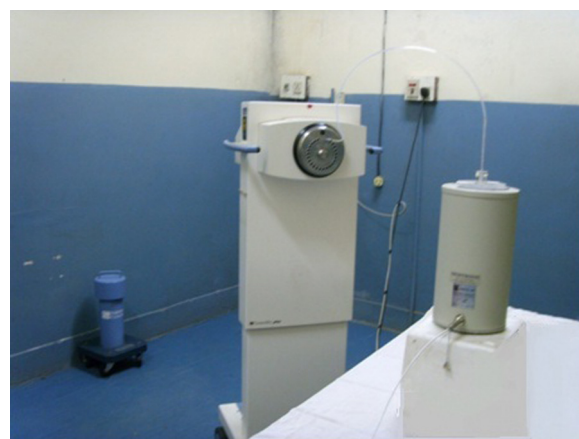
Fig. 1 – RAKR measurement set-up with well-type re-entrant chamber.
