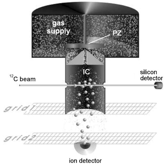
Fig. 1 – Schematic view of the Jet Counter.
