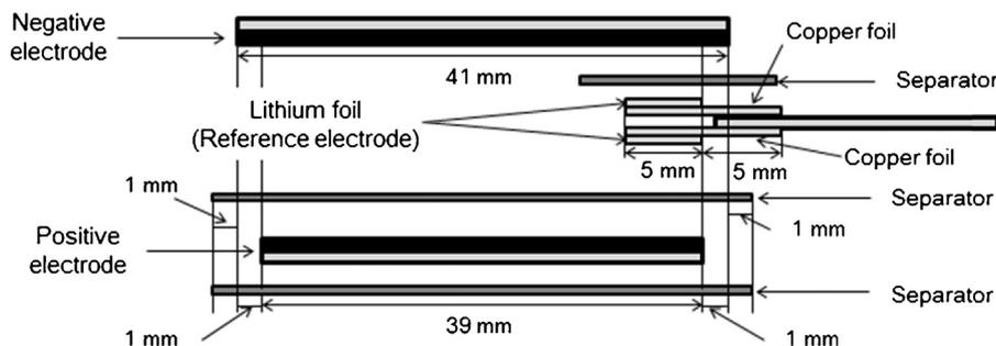
Fig. 1. Schematic illustration of the Li-ion secondary cell incorporating a reference electrode.
