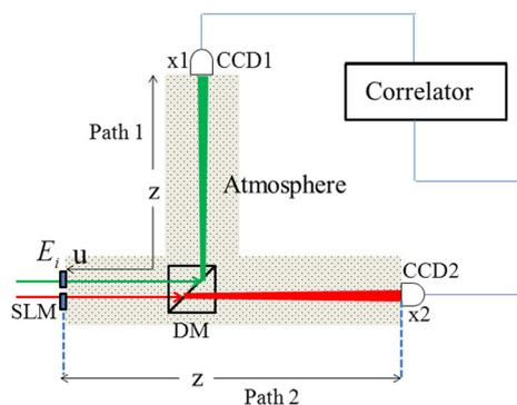
**Fig. 1.** The schematic for correlation between intensity fluctuations with two-wavelength in atmospheric turbulence. DM: dichroic mirror; SLM: spatial light modulator.
