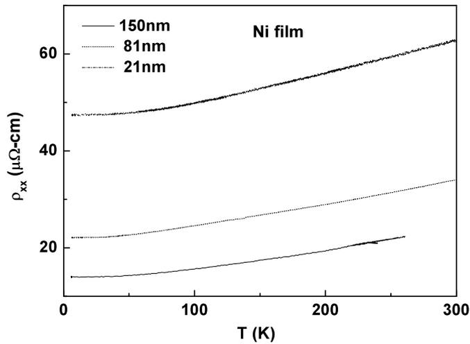
Fig. 1. The temperature dependences of Ni films with different thicknesses.
