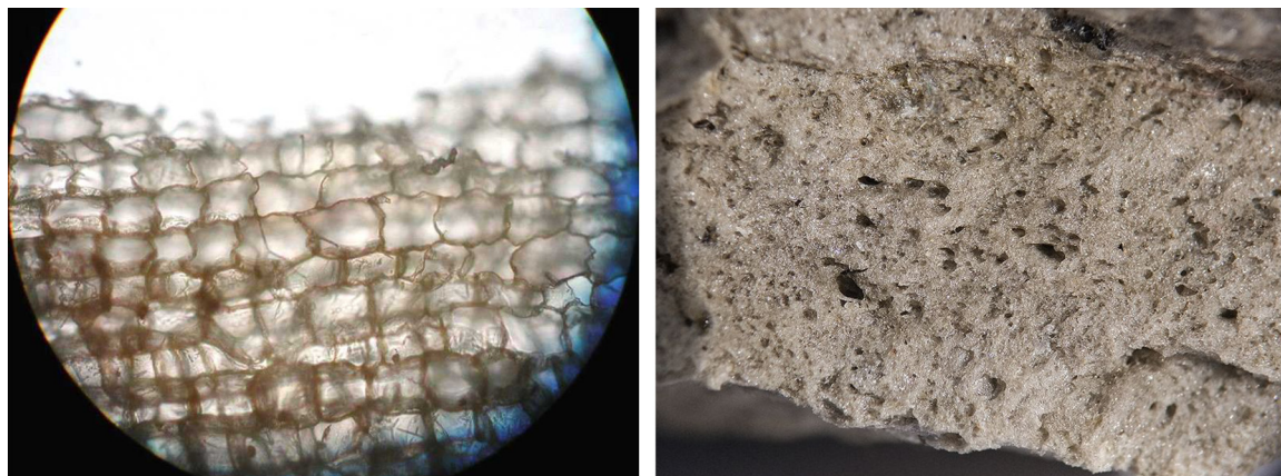
Fig. 1. (Colour online.) Microstructure of natural cellular and foam material. (a) Cork microstructure “à la Hooke”. Hooke [2] was the first to identify the cellular structure of cork. From D.B. Fankhauser [4]. (b) Pumice stone with a foam structure. Density may be as low as 0.25 \text{ g/cm}^3 . From Benjamin 444 [5].
