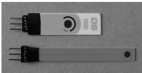
Fig. 1. Commercial electrode (DRP-110CNT-GNPE) above, screen printed carbon electrode (SPCE) below.
