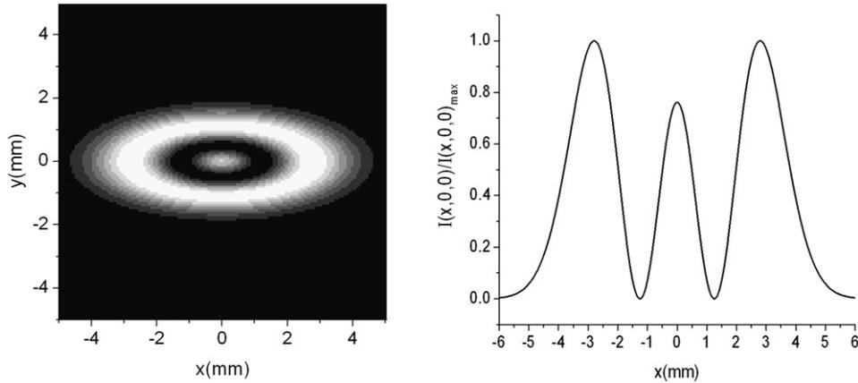
Fig. 1. Contour graph of the 3D-normalized irradiance and cross line ( $y = 0$ ) of an anomalous hollow beam with  $w_{0x} = 2.5$  mm and  $w_{0y} = 1$  mm.
