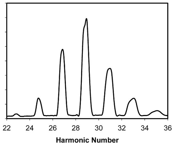
**Fig. 1.** XUV spectra emitted from argon at 25 Torr for a focus positions at the exit pinhole of the gas cell.
