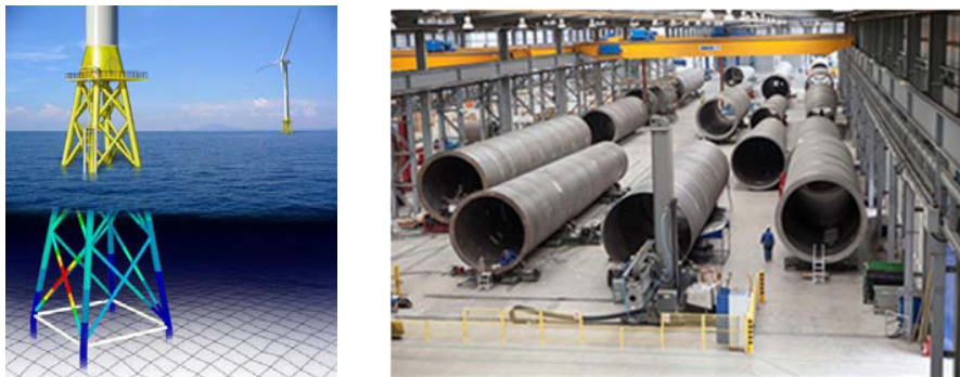
Fig.1 Offshore foundation jacket structure and windmill tower fabrication, (Mabey Bridge).
