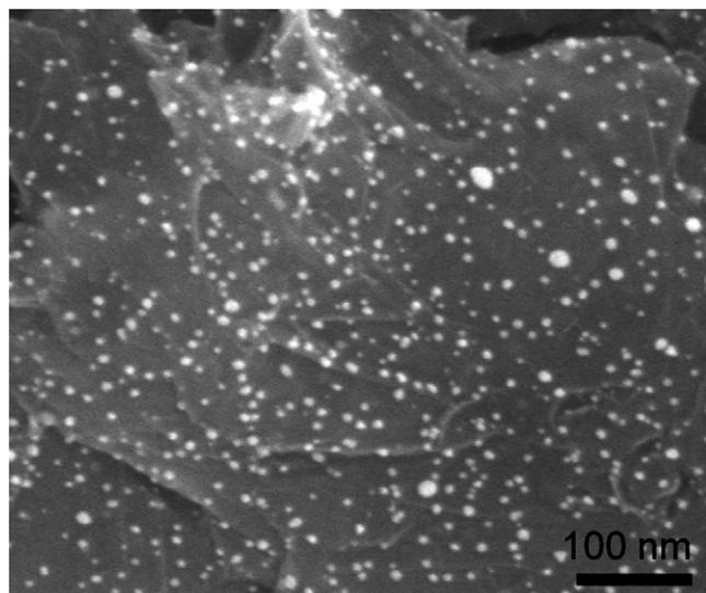
Fig. 1. SEM image of AuNPs/graphene/GCE.
